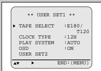
If you wish to use the tape counter to display the time remaining on a cassette, you must indicate the type of cassette inserted.
