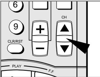
Select the channel by pressing the CH buttons (▲ or ▼) on the remote control.
