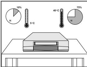
Do NOT expose the VCR to extreme temperature conditions (below 5°C(41°F) and above 40°C(104°F) or to extreme humidity conditions (less than 10% and more than 75%).
