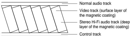
Hi-Fi audio recording and reproduction are available only from the Hi-Fi audio track, while the normal audio track provides normal audio.
