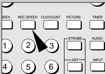
To record a cassette: Press the REC.SPEED button on the remote control, until:
