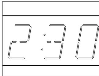
Press REC several times until the required recording time is displayed.
