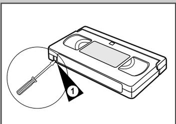
Video cassettes have a safety tab to prevent accidental erasure. When this tab has been removed, you cannot record on the tape.
