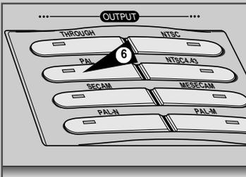
*You can convert the signal recorded on a tape to another format on a second tape.*
