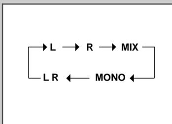
*You can select the mode in which the sound is reproduced on the LINE and AV outputs. The following options are available.*
